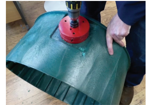
Drill holes into flat areas on risers.
